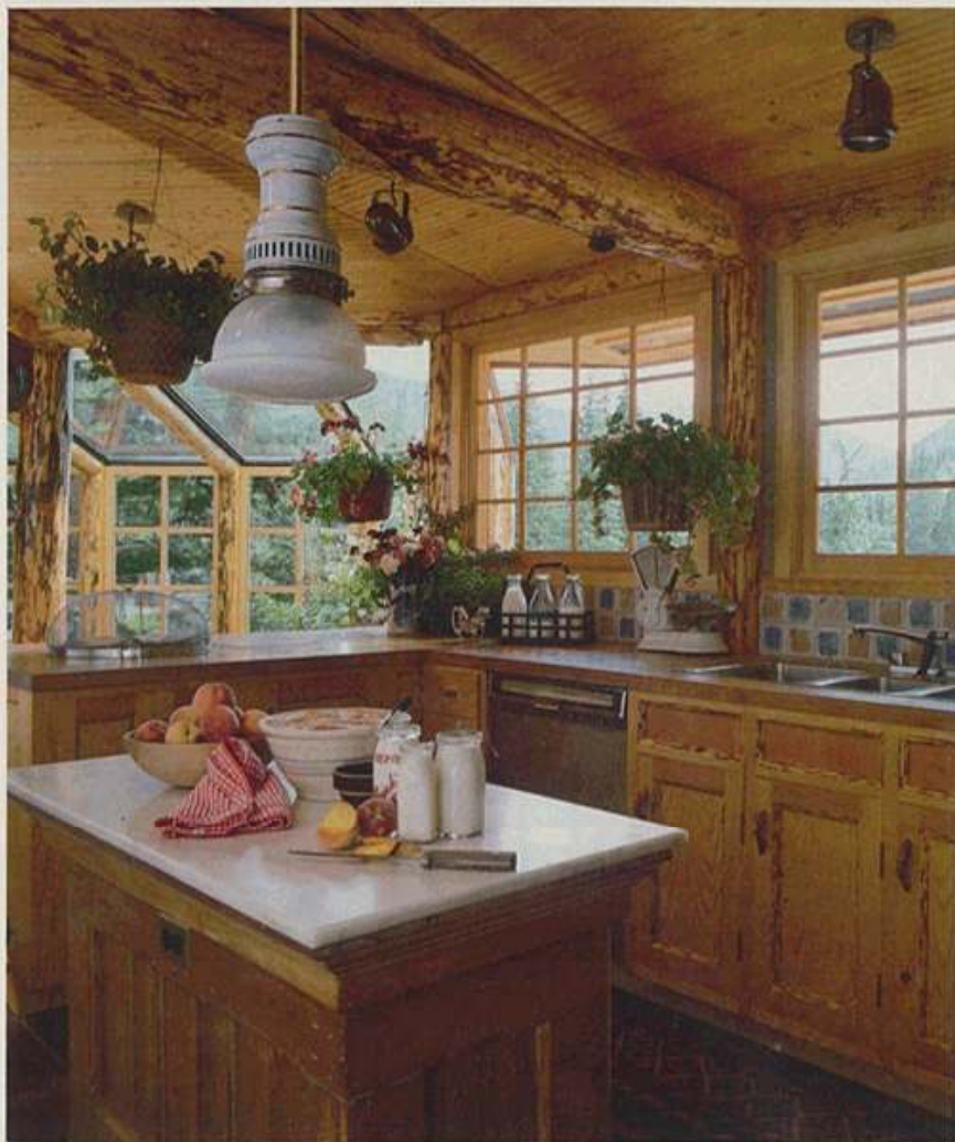
▲ The large kitchen is simultaneously rustic and thoroughly modern, belying the fact that plumbing and electrical work present special challenges in a solid-walled log home. Every piece of timber must be pre-drilled for wiring before assembly—no afterthoughts. Plumbing vents must rise through special furred-in “plumbing walls.”
